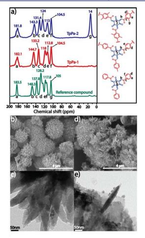
Figure 3. (a) Comparison of the <sup>13</sup>C CP-MAS solid-state NMR spectra of **TpPa-1** (red), **TpPa-2** (blue), and the reference compound 2,4,6-tris[(phenylamino)methylene]cyclohexane-1,3,5-trione (green). (b, d) SEM and (c, e) TEM images of (b, c) **TpPa-1** and (d, e) **TpPa-2** showing the nanoflower morphology.
